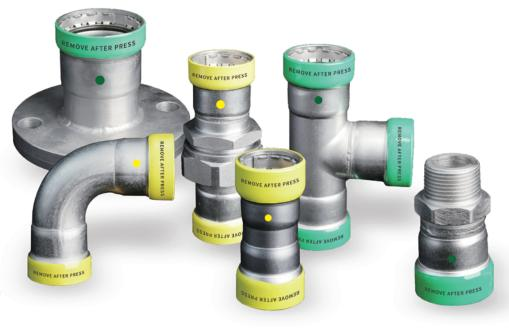
Carbon Steel fittings are for non-potable plumbing, natural gas, and LPG systems, designed to be used with schedule 10 to 40 Carbon Steel Pipe. Colour coded dots on the fitting indicate whether it's for non-potable water or gas.
